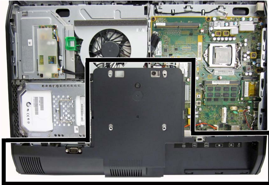
Figure 6-17 Lower panel location
